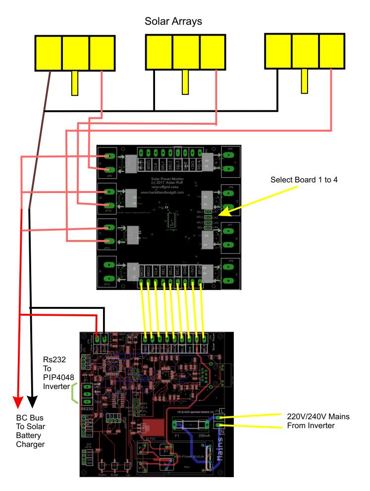
Solar Array Power Monitor With Serial Interface to MPPSolar PIP4048 Offgrid Inverter/Charger © 2018, Aidan Ruff
